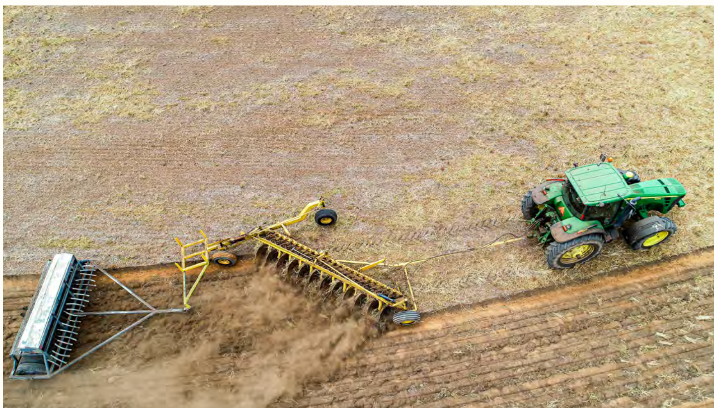
Plozza plough in action west of Kojonup in spring with a summer cover crop being sown from a trailing seed box to mitigate erosion.
